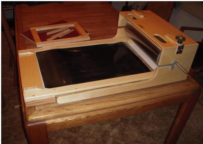
5. **Appearance:** It just looks nice! It is made primarily from oak, maple, and Baltic birch plywood with a Formica-covered 1-½" thick MDF platen. It is a satisfying and attractive piece of equipment to use. Since I am a cabinetmaker, I build this as a nice piece of woodworking, not as an industrial piece of machinery. Who says shop equipment has to look grey/black, heavy-duty, cast iron? Like the book-binding equipment I build, I take pride in the overall look and finish
