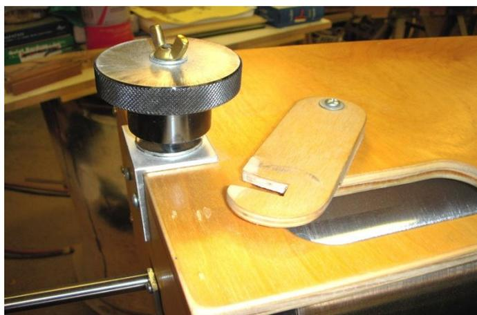
The black knobs on the top adjust the height of the cylinder. The wing nuts lock the knobs in place to keep them from changing height during the printing process.
