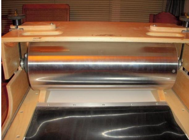
The cylinder weights about 50 lbs. How this amount of weight will make a satisfactory print depends on many factors, including how much type the cylinder contacts at one time. I have found that this is satisfactory without packing.
