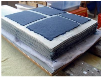
Post ready for pressing
